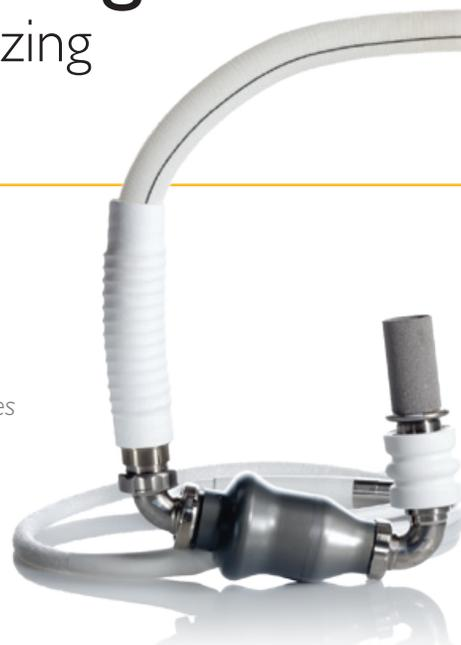
ascending aorta. The pump is axially configured, with blood flowing past the rotor parallel to the axis of rotation, allowing for a smaller size and weight compared to earlier devices and eliminating the need for a blood reservoir. Open-flow paths also help to maximize washing of the pump and conduits, contributing to the lowest published stroke and thrombosis rates among continuous flow LVADs.<sup>3</sup>
